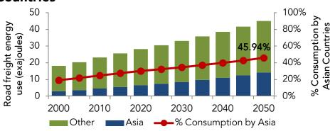
It is estimated that by the year 2050, energy use from medium and heavy freight trucks worldwide would be 45 Exajoules, growing 148% from 2000 levels at 18 Exajoules (WBCSD, IEA. 2001). Consumption of fossil fuels results to emissions of air pollutants such as particulate matter, Nitrogen oxides, Carbon monoxide, Volatile organic compounds, lead particles and Sulfur oxides.
